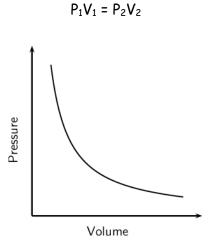
• The graph above shows the inverse relationship between pressure and volume of an ideal gas at constant temperature.
