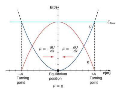
The total energy of a system undergoing SHM is defined by
