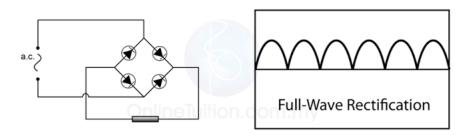
• Smoothing can be done with a capacitor to reduce the variation of the output voltage and current.
