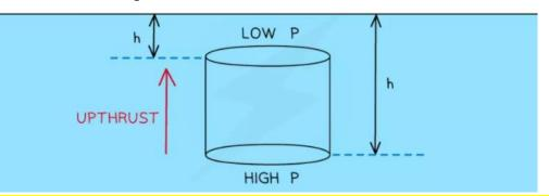
Archimedes' principle states that an object submerged in a fluid at rest has an upthrust equal to the weight of the fluid displaced by the object.
