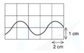
• The period of the wave can be determined from the time based (how
