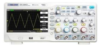
• Below is an example of a CRO display with the x-axis being time and y-axis being voltage
