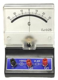
• The arrow on a galvanometer deflects depending on the amount of current passing through.
