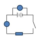
Label the voltmeter and ammeter. The figure above shows an electrical circuit with a 20  $\Omega$  resistor.
